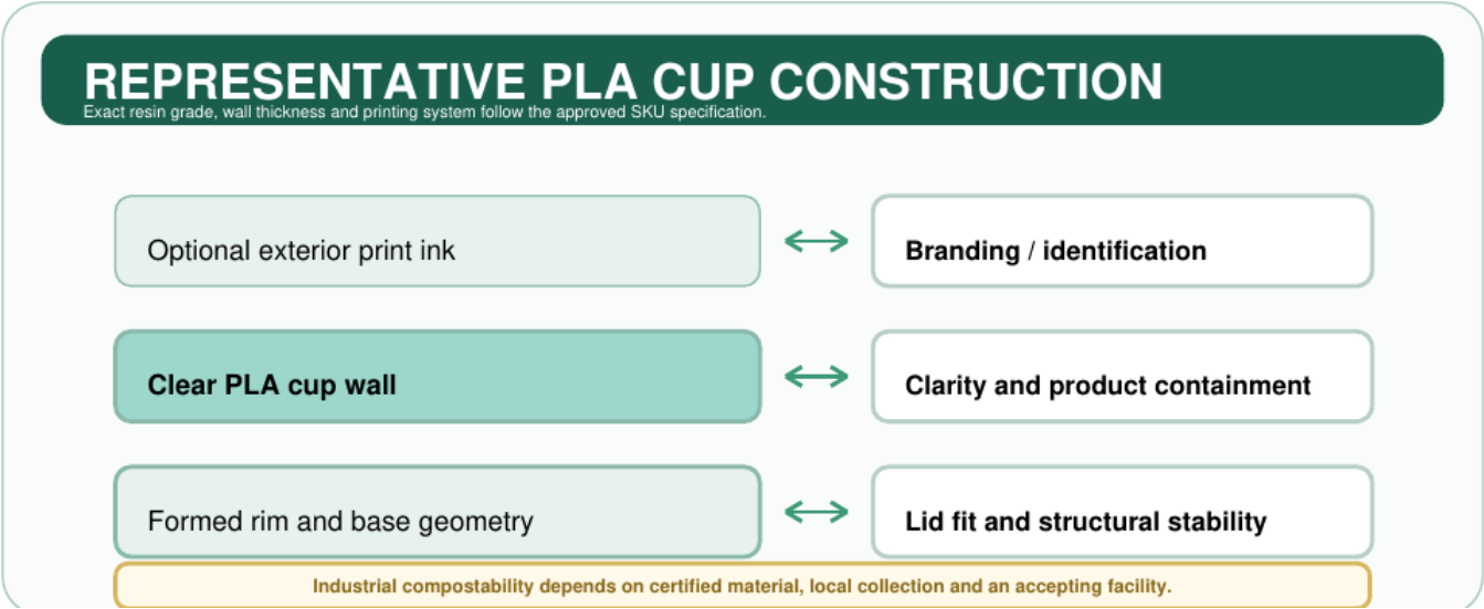
Representative PLA cup construction. Exact resin grade, wall thickness and printing system are confirmed in the approved SKU specification.
